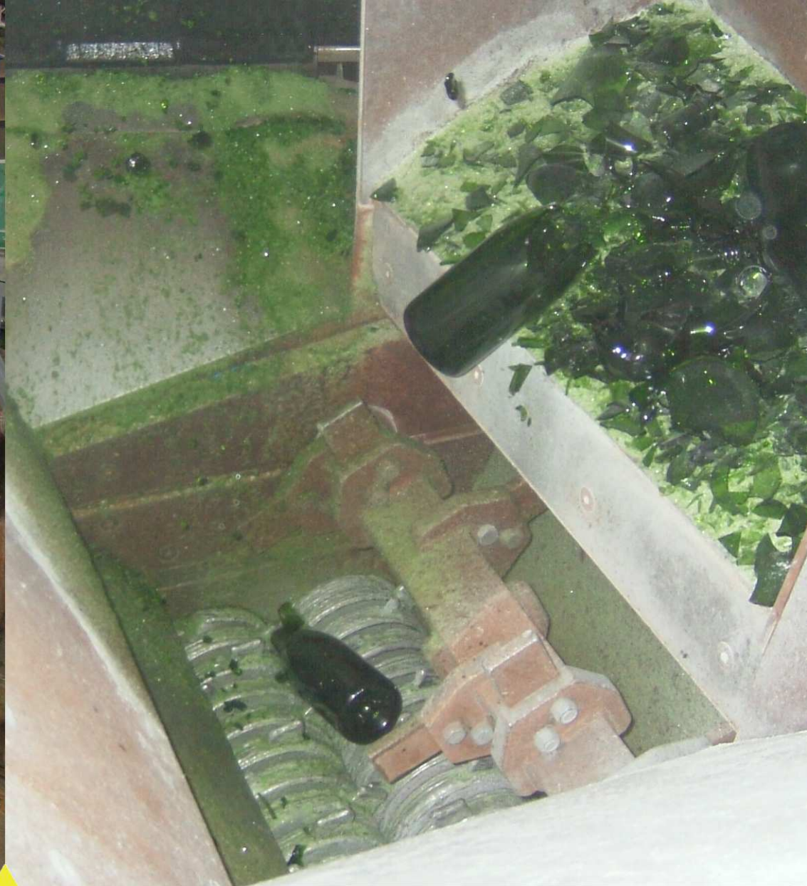
Glass bottle crushing unit toothed roll crusher type C200x800
